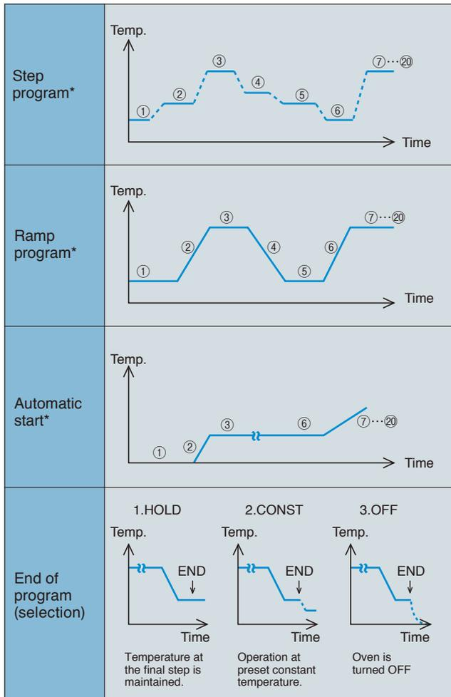
\* The number of repetitions of a program can be preset between 1 and 999. Stepwise damper setting is possible using an optional automatic damper. Guarantee soak function, whereby the timer is used to maintain a preset temperature for a preset length of time, can also be performed.
