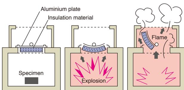
In case an explosion occurs inside the test chamber, as shown in the above image, insulation material is bent and blown upward together with the aluminium plate to the metal screen at the top of the chamber.
